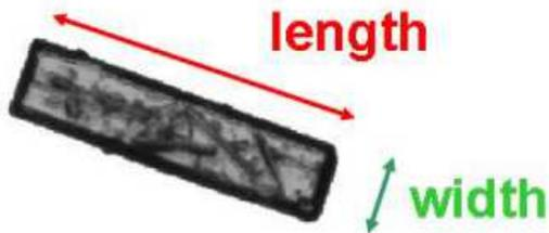
$$\text{Circularity} = \frac{2 \times \sqrt{\pi \times \text{Area}}}{\text{Perimeter}}$$
